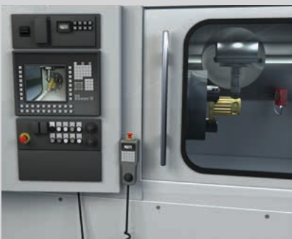
Rear area monitoring in CNC machine
